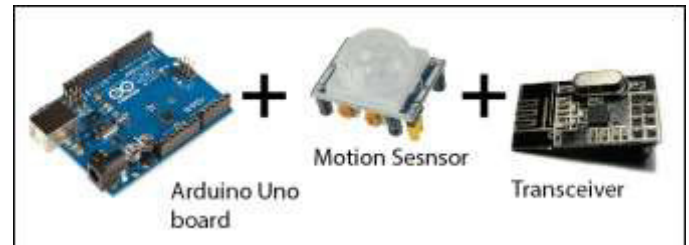
Figure 3. Arduino-board (Child Node) with Motion Sensor
