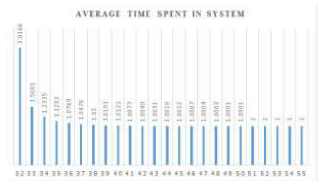
Figure 5. Average time passengers spent in immigration system with different number of counters.
