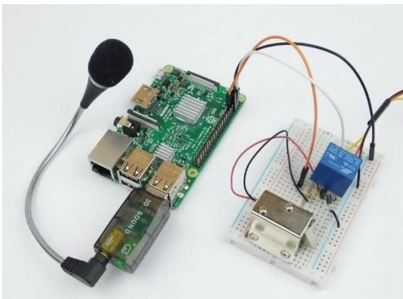
Figure 4. Hardware Use in Voice Activated Entrance System
