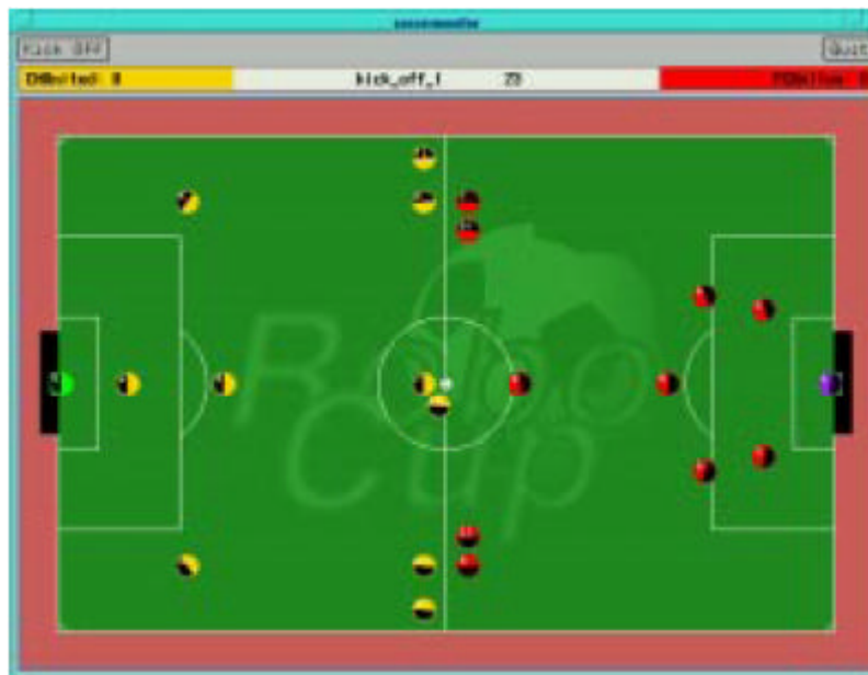
Fig 2: The soccer server display. Each player is represented as a two-halved circle. The light side is the side towards which the player is facing. All players are facing the ball, which is in the middle of the field. The black bars on the left and right sides of the field are the goals.
