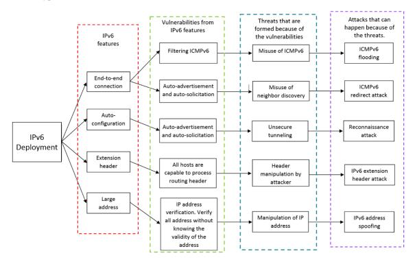
Figure 1. Potential attacks that can be resulted from threats and vulnerabilities of IPv6 features
