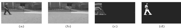
Figure 2: Mixture of Gaussian modeling for background subtraction. (a) Image from a sequence in which a person is walking across the scene (b) The mean of the highest-weighted Gaussians at each pixel position. These means represent the most temporally persistent per-pixel color and hence should represent the stationary background. (c) The means of the Gaussian with the second-highest weight; these means represent colors that are observed less frequently.
